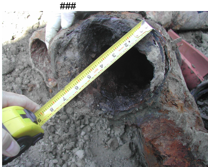
This 6" inch pipe had heavy build up where an 1-1/2" + of pipe diameter was lost on each side
